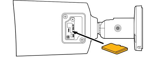
NOTE: Maximum SD Card size supported: Up to 1TB micro SD / FAT32. When inserting the SD card into the card slot, the SD card's contacts should be facing upward, as shown in the diagram.
